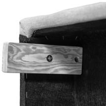
4. Place the back to be assembled on the assembly aid.
