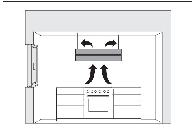
The device is used in recirculated air mode.
