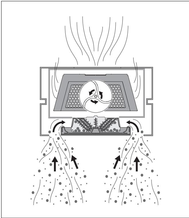
Cooking vapours are drawn through a gap and into the hood where they are accelerated and routed through bends.
