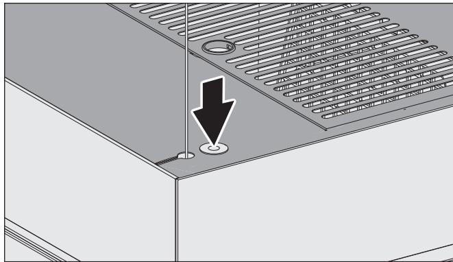
The pairing button is located on the top of the device.
